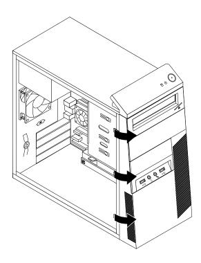
Figure 10. Removing the front bezel
